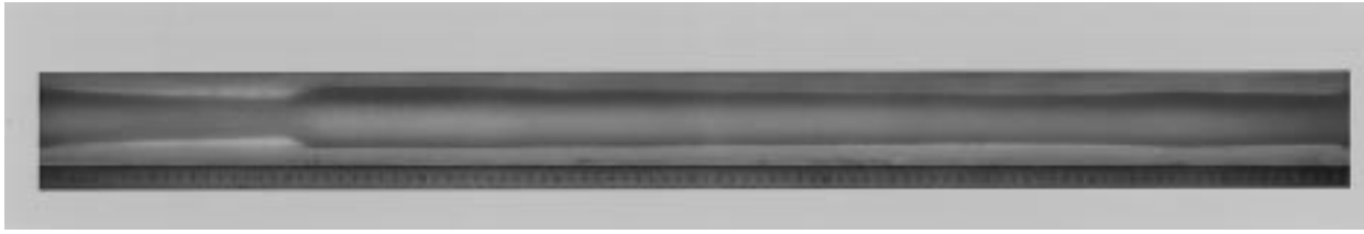
Fig. 6. Ice layer with two waves at Re_D = 10,000 , B = 10 , N = 0.5 .
