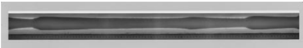
Fig. 7. Ice layer with three waves at Re_D = 10,000 , B = 18 , N = 0.5 .
